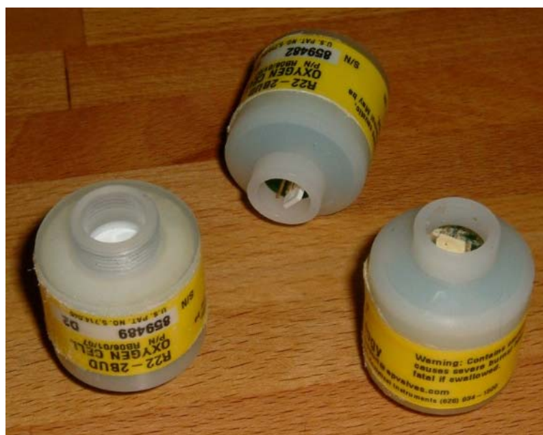
Fig. 1 – Electro-galvanic fuel cells used for diving applications
