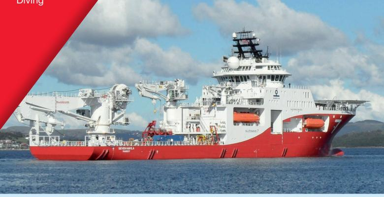
The *Seven Falcon* is one of the most advanced diving vessels in the world, featuring a 24-man twin bell saturation diving system operationally rated to 300m, and a heave compensated 250t crane.
