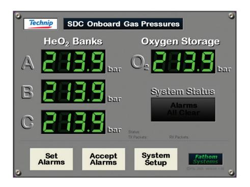
Audible and visual alarms alert the supervisor to any loss of pressure and allows appropriate remedial action to be taken. The iCG can be supplied as a stand-alone system comprising a bell-mounted pod, topside touch-screen panel PC, topside interface unit and interface cables.
